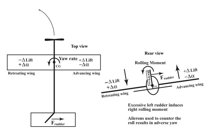
Figure 1. Anatomy of a base-to-final stall-spin.
