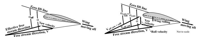
**Figure 2.** The effect of yaw rate on angle of attack.
